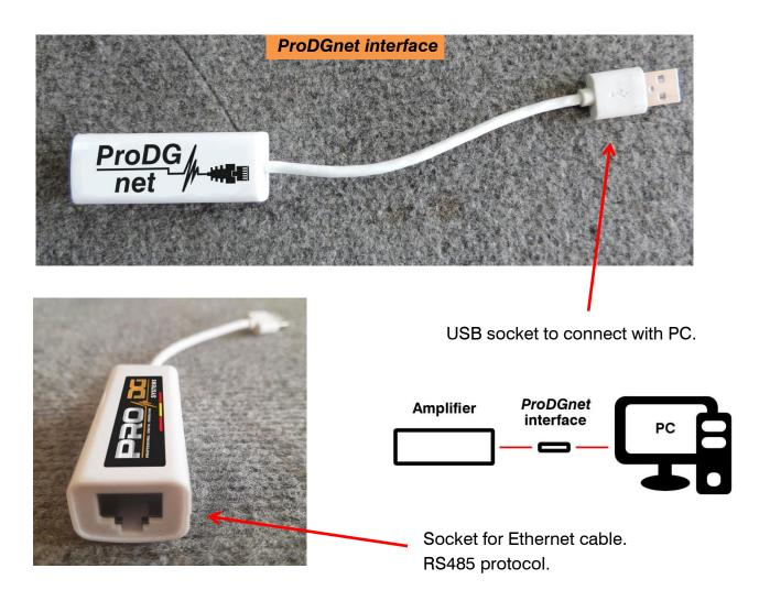
Below is a **guide for use** and information on the different menus of the *ProDGnet software*, which we can see **when we connect the DSP module of the unit to the PC**, through the ProDGnet interface:
